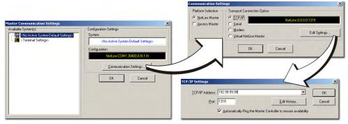
FIG. 31 Assigning Communication Settings and TCP/IP Settings
